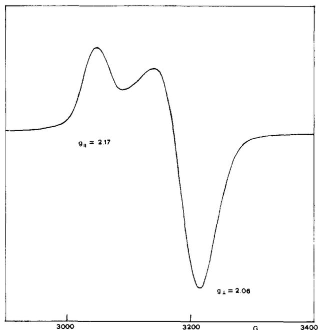
Figure 4. X-Band (9 GHz) ESR spectrum of Ni([12]aneN<sub>4</sub>)<sup>3+</sup> in acetonitrile solution, 0.1 M in Bu<sub>4</sub>NBF<sub>4</sub>, frozen at 77 K.
