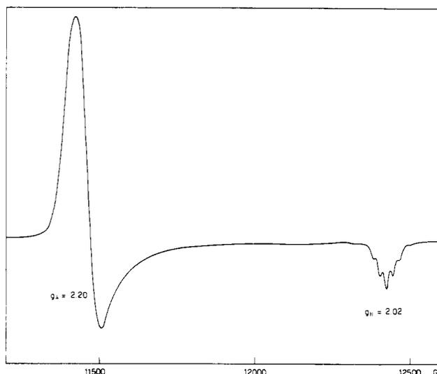
**Figure 2.** Q-Band (35 GHz) ESR spectrum of  $\text{Ni}([13]\text{aneN}_4)^{3+}$  in acetonitrile solution, 0.1 M in  $\text{Bu}_4\text{NBF}_4$ , frozen at 77 K.
